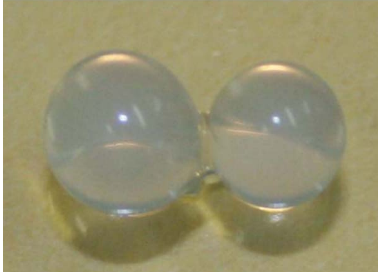
Fig. : 1. Magnified photograph (12.5 x) of \alpha -amylase entrapped inside calcium alginate beads using Kodak digital camera
